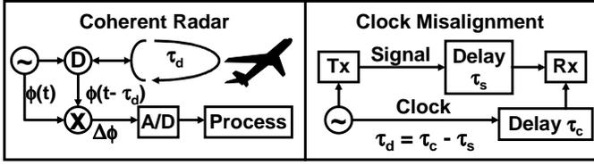
Figure 5. Systems that have a delay  $H_s(f)$ .
