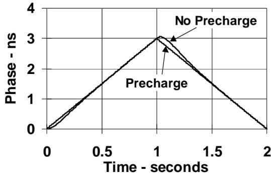
Figure 8. Measured PLL Performance with and without Precharge.
