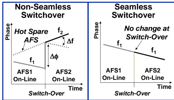
Figure 1. Seamless vs Non-Seamless Switchover.
