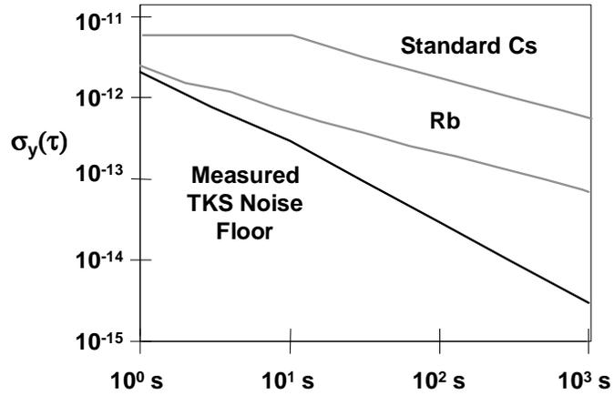
Figure 6. Measured Performance of TKS Phase Measurement System.
