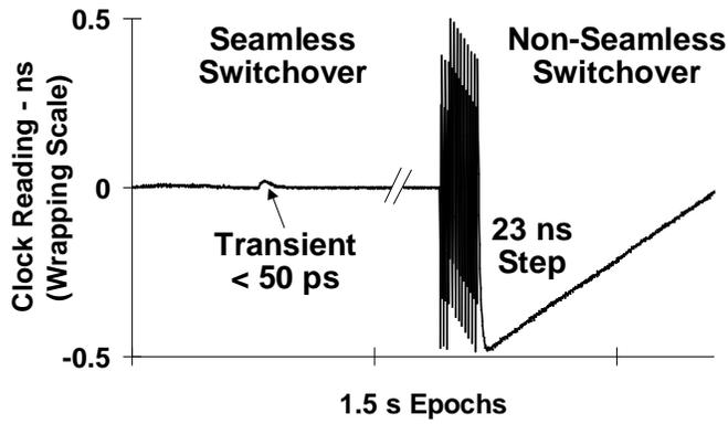
Figure 10. Measured Results for Seamless vs Non-seamless Switchover.
