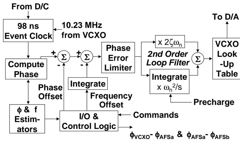
Figure 7. Phase Lock Loop Processor and Event Clock.
