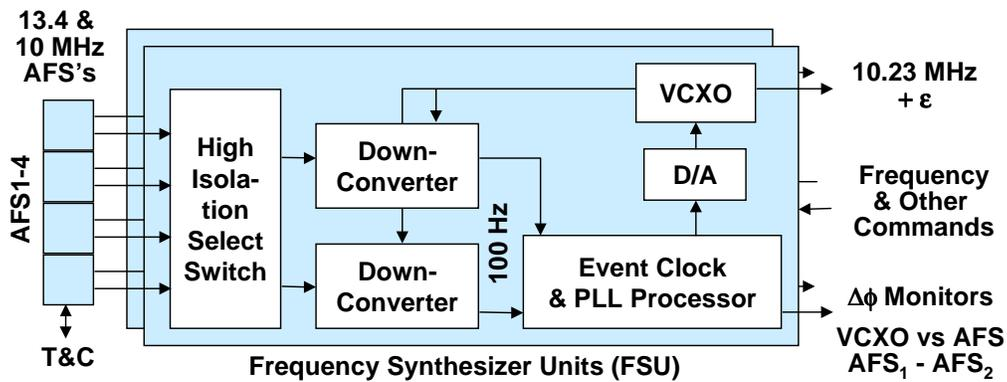
Figure 2. Redundant AFS Time Keeping System.
