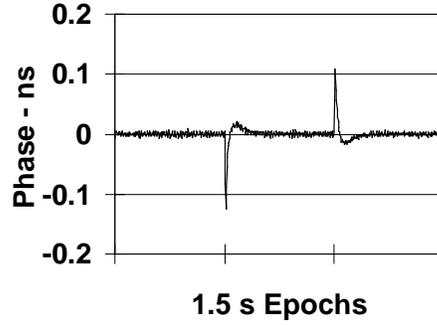
Figure 9. Measured Deviation from Ideal Frequency Step (with Precharge).
