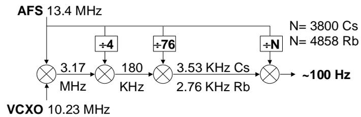
**Figure 5. Typical Downconverter Configuration.**
