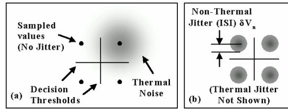
Figure 6. ISI and BER degradation: (a) Ideal system. (b) System with ISI.
