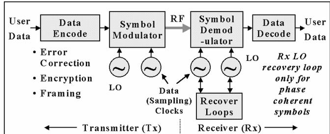
Figure 7. RF carrier digital communications system .
