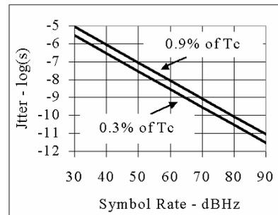
Figure 12. Typical decision epoch jitter requirements vs symbol rate.
