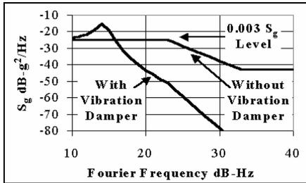
Figure 10. Typical commercial aircraft vibration levels [9].
