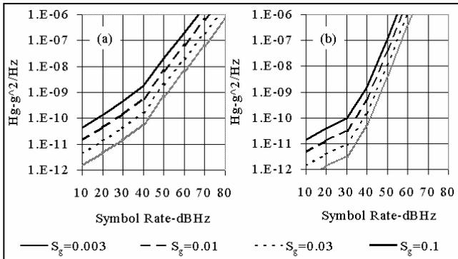
Figure 11. LO g-sensitivity requirements as a function of symbol rate for  $0.25^\circ$  of allocated phase jitter and 10 GHz  $f_0$ : (a) without vibration damper and (b) with vibration damper.
