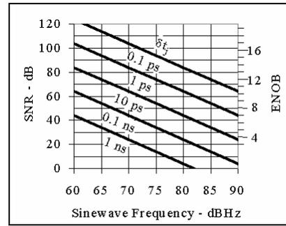
Figure 14. Effect of sampling clock jitter on A/D and D/A SNR and ENOB vs full scale sine wave frequency [10].
