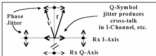
Figure 8. ISI caused by RF carrier phase jitter.
