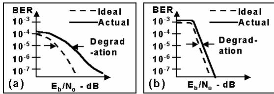
Figure 5. Typical BER vs  $E_b/N_o$  curves: (a) Uncoded. (b) Coded.
