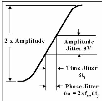
Figure 13. Impact of sampling clock jitter on digitized sine wave [10].
