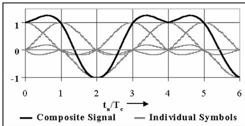
Figure 3. Digital transmission consisting of multiple shaped symbols.
