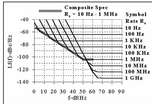
Figure 9. LO phase PSD curves for 0.5° of allocated phase jitter.
